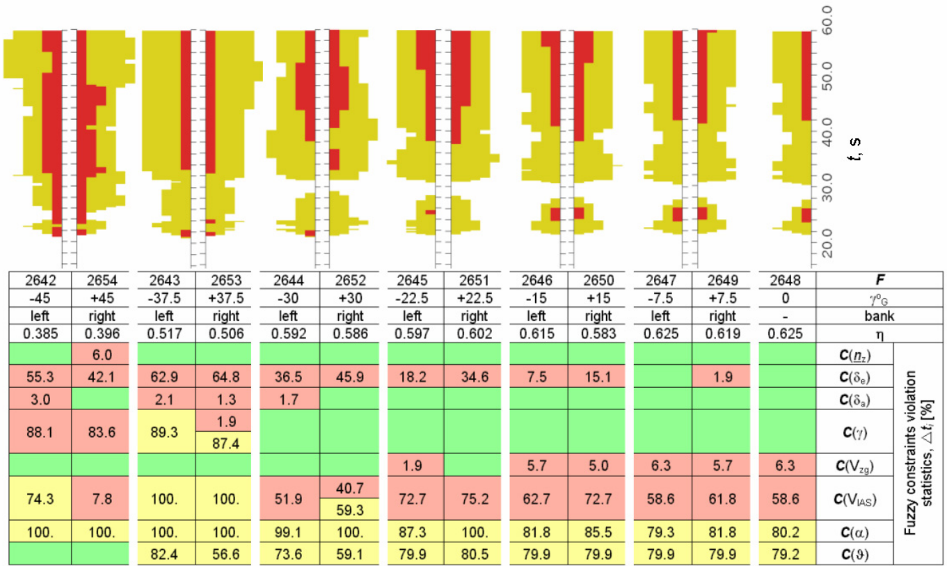
Fig. 8: Effect of magnitude and direction of bank on flight situation complexity – a sub-tree from situational tree T_{130} | \Gamma(\Phi_1 \times \Phi_2) : “Takeoff and initial climb, \gamma_G = var , \Theta_G = 16^\circ , \gamma_G \in \{-45^\circ, \dots, +45^\circ\} ”, where T_{130} = \{F_{2551}, \dots, F_{2680}\} , \Phi_1 = \Theta_G , \Phi_2 = \gamma_G
